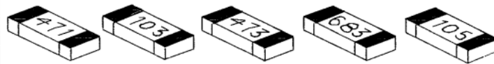
The 5 chip resistors used in this project are: 470R, 10k, 47k, 68k and 1M.
